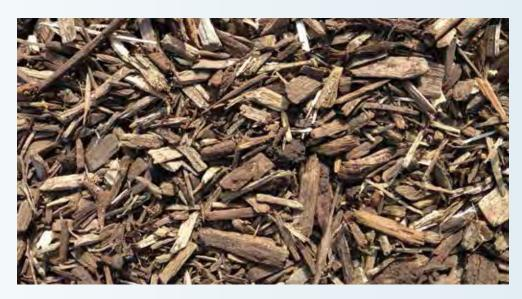
Filtrexx products are designed to Mimic Nature®—we use an aged composted FilterMedia™ inside a tubular mesh to harness nature's design principles of containment, filtration, retention, detention, energy dissipation, and vegetation establishment. As stormwater flows through the Soxx sediment and soluble pollutants are removed by:
